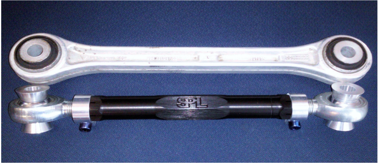
Illustration 1: Try to match length of new link to that of old, center to center of the bores. This will enable you to drive to your alignment shop.
