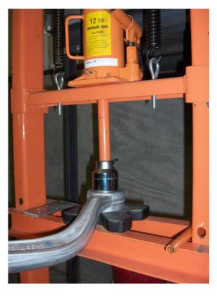
Measure bushing bore of knuckle and measure diameter of new bushing with caliper. Confirm that new bushing is between 2/1000 - 4/1000 inch larger than the bore.
