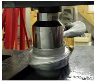
Be sure to have the arm level so the driver/socket can press out the bushing straight to avoid binding. Once square, press out the old bushing. Clean the bore of the arm, and smooth any knicks or burrs. The same socket can then be used to drive in the new bushing. Again, make sure to align the driver and bushing to go in straight and not bind.
