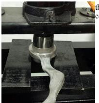
the new bushings will alter the alignment compared to the stock alignment.
