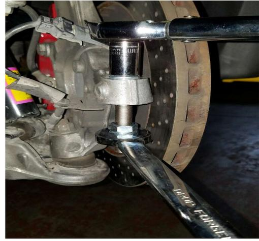
Remove the two silver colored nuts. Install supplied stainless steel spacers to adjust bump steer. You will want to try to make the angle of the tie rod set up match the angle of the lower control arm. The lower the car, the more spacers you will use. (See pictures for various combinations.) Test and adjust from there. Install locking nut on bottom. This nut will take some effort to thread (about 20 ft-lbs of torque) as it is a metal crimping/locking nut. **TORQUE TO 80 ft-lbs.**
