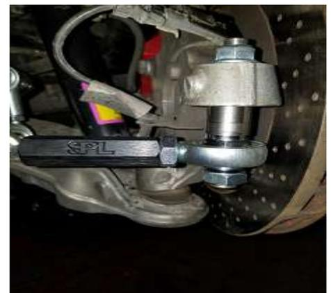
Check for binding or any problems by rotating steering wheel lock to lock with car sitting on ground. Check that the spherical bearing does not bind (the edge of the ball bearing hitting or close to hitting the housing) under any situation as shown in the picture below. After installing, run the suspension and the steering rack from lock to lock through its travel to make sure there is no contact between the arms.
