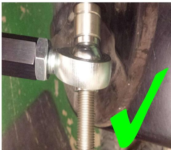
Note that the inner tie rod end can rotate freely, so the picture on left is not binding even though the edge of the ball is touching the housing. If uncertain, try rotating the inner tie rod by using a wrench on the hex part of the inner tie rod.
