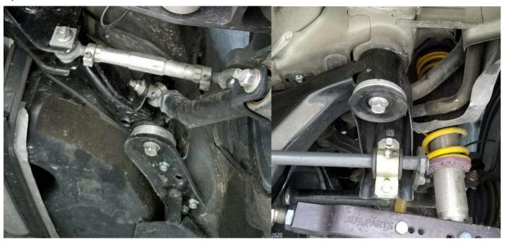
*Optional*: The supplied rubber isolators can be installed between the chassis and the subframe bushing to help dampen some noise.
