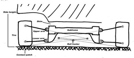
The following diagram shows the subframe raised closer towards the chassis (no more gap between subframe and chassis), and the ride height lowered the same amount. The roll center position is un-changed.
