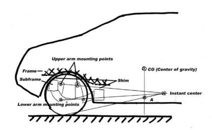
The following diagram shows what happens when you raise the subframe closer to the chassis. For this example, we are comparing what happens to the anti-squat when the ride height remains the same. When the subframe is raised, the rear "instant center" is raised as well, that moves point A up and increases anti-squat.
