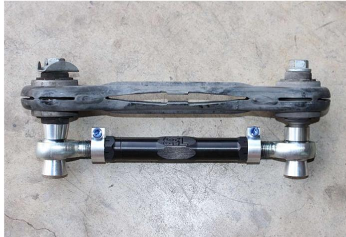
4. Install the SPL Parts Arm using the OEM hardware. Please ensure the Tapered Stainless Steel Spacer (2) provided mates up with the tapered section of the knuckle. Tighten the nuts to **73.7 ft. lbs.** (100 N/M) at both ends. **DO NOT OVERTORQUE!** *SPL Parts is not liable for any issues due to overtorque.*
