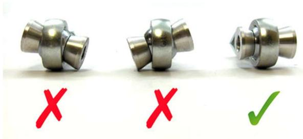
5. Once installed, ensure that both of the FK Rod Ends (4, 5) are centered and have full articulation. Lock them in place by tightening the Blue Titanium Socket Head Cap Screws (7) with a 3/16 allen wrench to **150 IN. lbs.**
