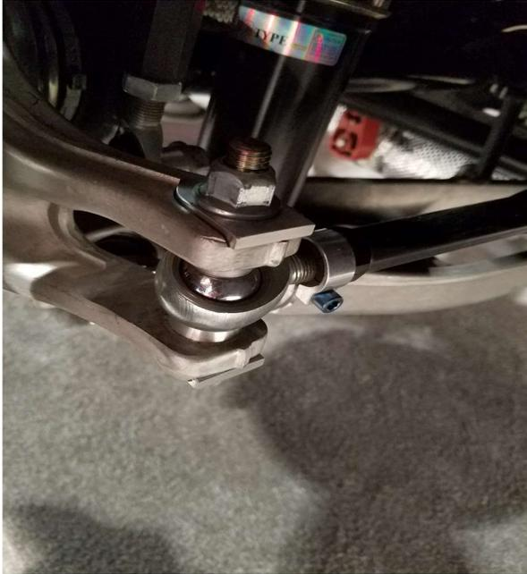
3. Install the provided Eccentric Lockout Washers (8) in the subframe. They should fit between the two grooves in the subframe and prevent the bolt from moving.
