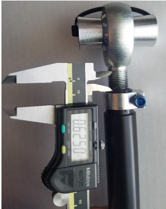
Loosen the Aluminum Clamps (6) on both ends of the Turnbuckle. Turn the Turnbuckle so as to thread in/out the FK Rod End (spherical bearing side). Threading in/out the FK Rod End will in turn thread out/in the Turnbuckle on the chassis side.
