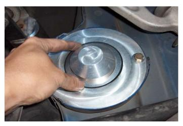
5. Place the supplied Swift spring thrust washer on the upper perch (carbon washer on top against the perch, then steel washer on top of the spring), and hold the spring in place on the upper perch.
