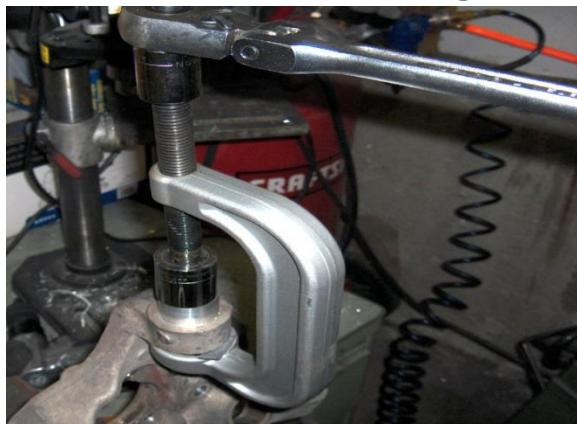
1. Press out the stock bushing using an appropriate bushing press and driver.
