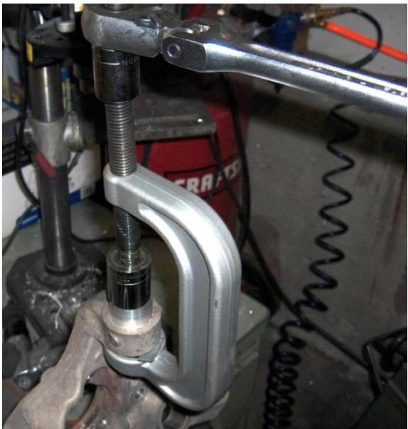
7. Press in the new bushing completely with an appropriate press and driver.
