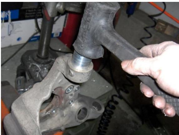
6. Lightly tap the new SPL Parts bushing in place to start, making sure the bushing is square against the bore.
