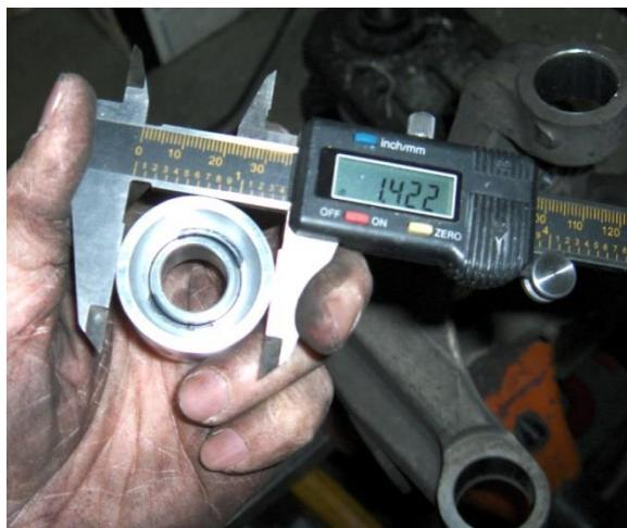
3. Measure the bushing bore of the knuckle.
