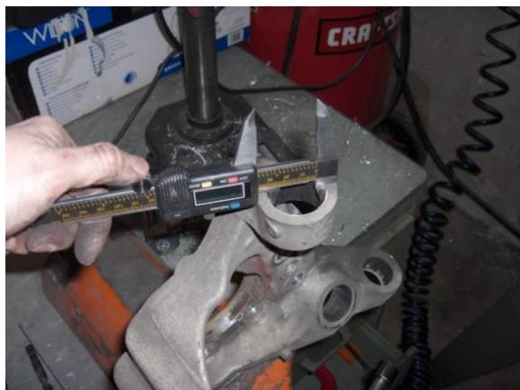
2. Clean the bore and file down any nicks in the bore as necessary.
