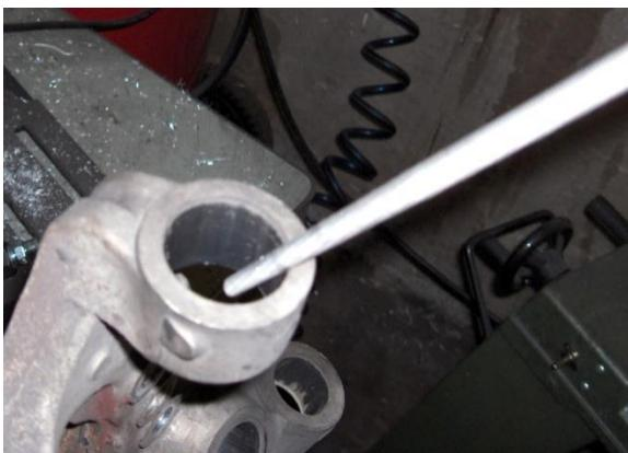
5. If the side of the knuckle which the new bushing goes in is not chamfered, use a round file to break the edge.
