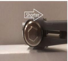
When all adjustments are finished, make sure the clamps are orientated downward to allow maximum clearance to the chassis.
