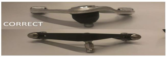
The images above show the correct way to determine what arm goes on what side of the vehicle. Match up the SPL arm with the OEM arm by observing the canted balljoint. This will allow proper articulation of the balljoint.
