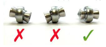
The advantage of the hybrid adjuster is that you can easily keep the rod end bearing centered during and after alignment. Make sure to keep the bearing centered as shown.
