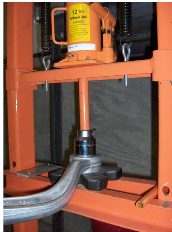
3. Measure the bushing bore of the knuckle and measure the diameter of the new SPL Parts bushing with a caliper. Confirm that the new SPL Parts bushing is between 2/1000 – 4/1000 inch larger than the bore.
